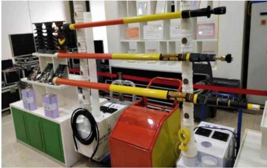
Primary equipment cleaning machine
